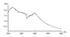
Figure 3 - Characterization of AgNPs with a peak at 400 - 420 nm.
