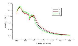
Figure 6 - UV-vis spectroscopy results showing concentration of leaf extract Vs. silver nano particles synthesis. (G-2:1, D-1:1, B-3:1).
