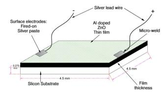
Figure 3. Schematic of CO gas sensing.
