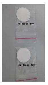
Figure 2. Sputtering target.
