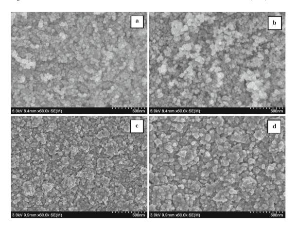
**Figure 11.** Microstructure of Al-doped ZnO thin films for grey theory predicted design at different annealing temperatures, (a) 350, (b) 400, (c) 450 and (d) 500°C.
