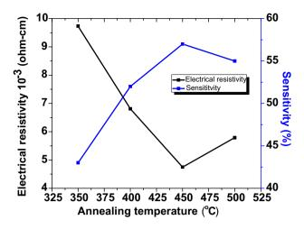
**Figure 8.** Resistivity and sensitivity plotted as a function of annealing temperature for Al-doped ZnO thin films.
