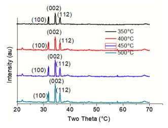
**Figure 10.** XRD pattern for Al-doped ZnO (1 wt.% Al) thin film for grey theory predicted design at different annealing temperatures, 350, 400, 450 and 500°C.
