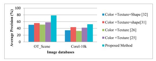
Fig. 5. Average precision rate of feature integrated methods [32],[31],[26],[25], and proposed method.
