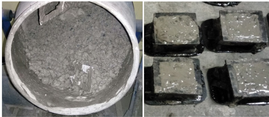
Figure 2: Geopolymer concrete at the time of mixing and casting.
