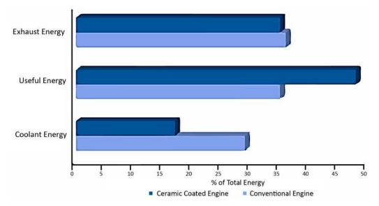
Figure 1. Property enhancement on the application of ceramic coatings in internal combustion engines.
