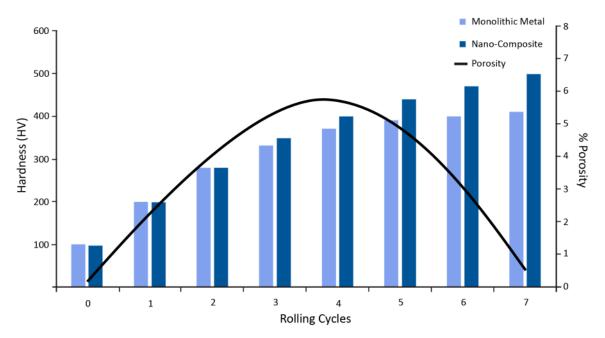
Figure 15. Hardness and porosity dependence on rolling cycles.
