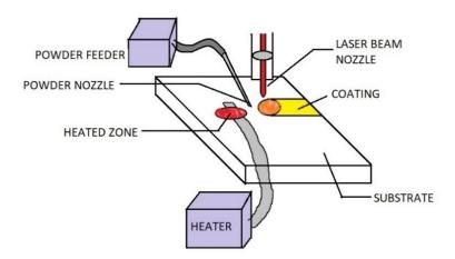
Figure 12. Pre-heating surface treatment.
