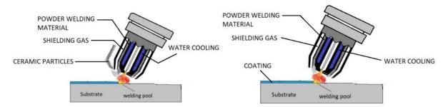
Figure 11. Synchronous Feeding (right) and Back Feeding (left) mechanisms.
