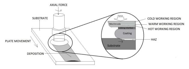
Figure 7. Schematics of friction surfacing.
