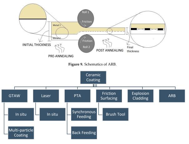
Figure 10. Processes and sub-systems for ceramic coating.
