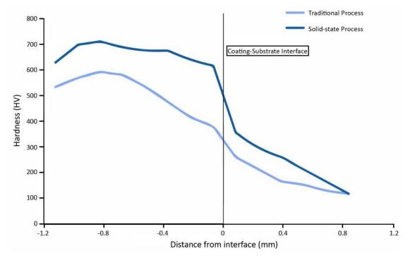
Figure 14. Distribution of hardness along with the depth of a sample.
