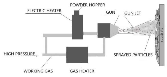
Figure 3. Cold spraying—a solid-state process.
