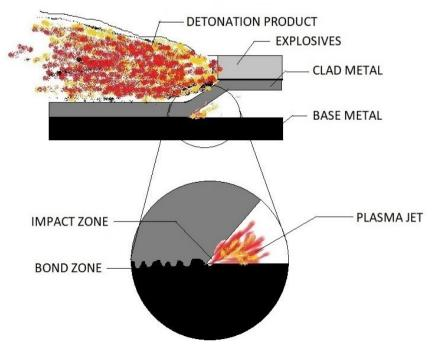
Figure 8. Explosion cladding.
