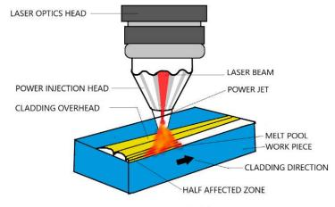
Figure 5. Laser cladding.
