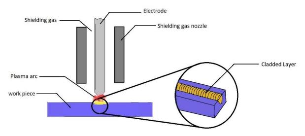
Figure 4. Schematics of gas tungsten arc welding (GTAW).
