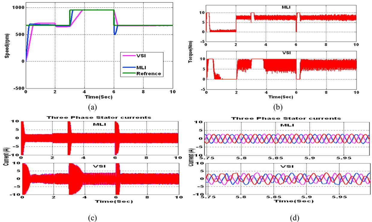
Fig. 5. MLI and VSI fed drive responses for change in speed (a) Speed (b) Torque (c) Stator current (d) Zoomed view of stator current
