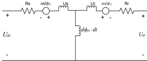
Fig. 2. Induction Motor circuit in d-axis
