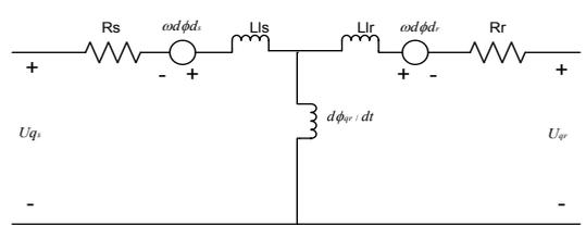
Fig. 3. Induction motor circuit in q-axis
