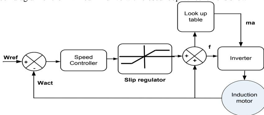
Fig. 4. Induction Motor closed loop speed control
