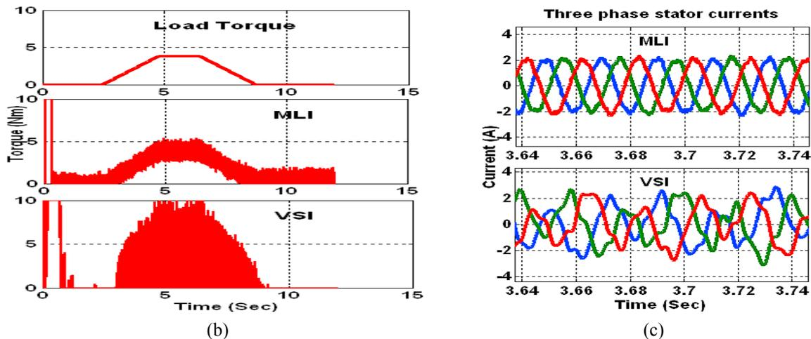
Fig. 7. MLI and VSI fed drive responses for trapezoidal change in load torque (a) Speed (b) Torque (c) Stator current
