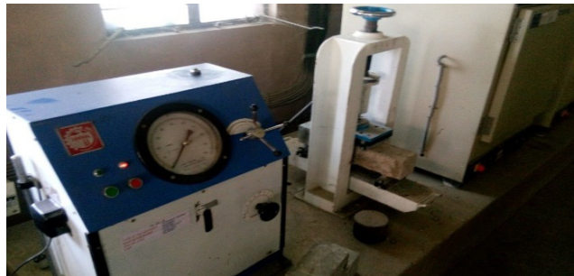
Figure 2. Flexural strength testing machine - third point loading arrangement.
