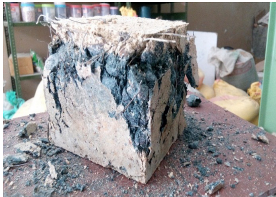
Figure 1. Geopolymer concrete specimen subjected to compression testing containing steel fibres.
