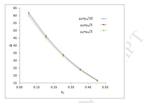
**Fig. 6:** Mass-flux Q variation versus aspect ratio  $\varepsilon_1$  for values viscosity ratio when  $\theta = 0.3$
