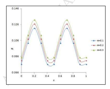
**Fig. 3:**Peripheral velocity  $u_f$  versus z profiles for values 6 when  $\mu_2 = \mu_1 / 10 \epsilon_1 = 0.2$
