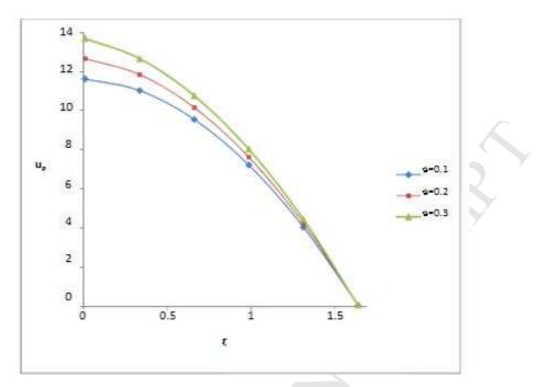
**Fig. 2:**Plug core velocity  $u_p$  versus r profiles for values  $\theta$  when  $\mu_2 = \mu_1 / 10 \varepsilon_1 = 0.2$
