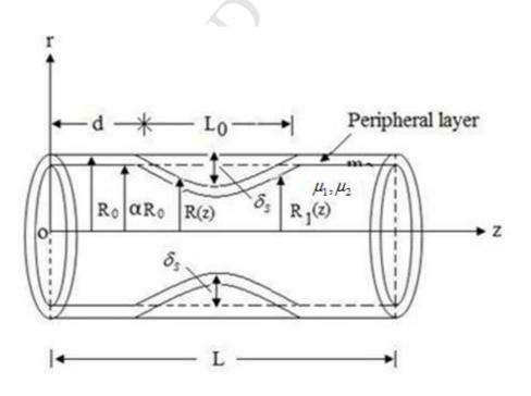
Fig. 1: Geometry of a stenosed artery with peripheral layer
