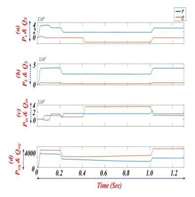
**Figure 8.** PV-STATCOM performance: **(a)** source powers (P&Q); **(b)** load powers (P&Q); **(c)** PV-STATCOM powers (P&Q); and **(d)** wind generator powers (P&Q).
