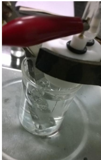
Figure 4. Photograph showing the hydrogen evolution at the working electrode during the TAFEL studies
