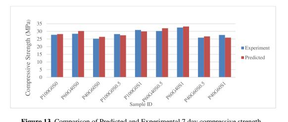
Figure 13. Comparison of Predicted and Experimental 7 day compressive strength.
