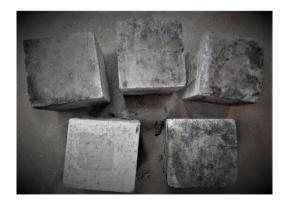
Figure 9. Cracked cubes in room temperature.
