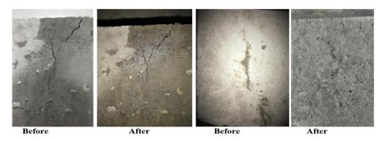
Figure 12. Cracks visibility before and after curing in a room atmosphere for 28 days.
