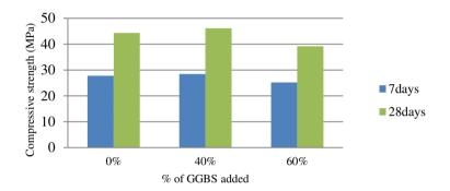
Figure 6. Graphical representation of compressive strength with various GGBS content.
