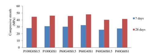
Figure 7. Graphical representation of compressive strength with various proportions of SAPs.
