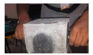
Figure 4. The test set up for Ultrasonic Pulse Velocity Test (UPV).
