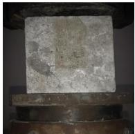
Figure 8. Application of compressive load up to first visible crack.
