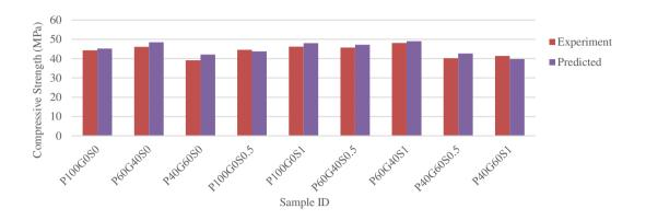
Figure 14. Comparison of Predicted and Experimental 28 day compressive strength.
