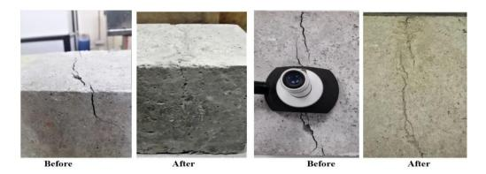
Figure 11. Cracks visibility before and after curing in water for 28 days.
