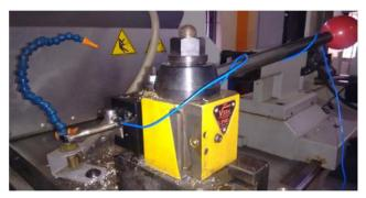
Figure 2. Arrangement of sensor on the boring bar.
