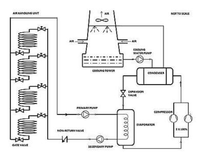
Figure 1. Schematic diagram of Chiller Plant
