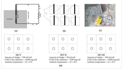
**Figure 1.** Single chamber single electrode MFC. (a) Circuit diagram of single cell of single chamber single electrode MFC. (b) Schematic representation of the circuit diagram of single chamber single electrodes MFC in series. (c) Photograph of the experimental setup of the combination of single chamber single electrode. (d) Schematic representation of the three different setups of MFC studied.
