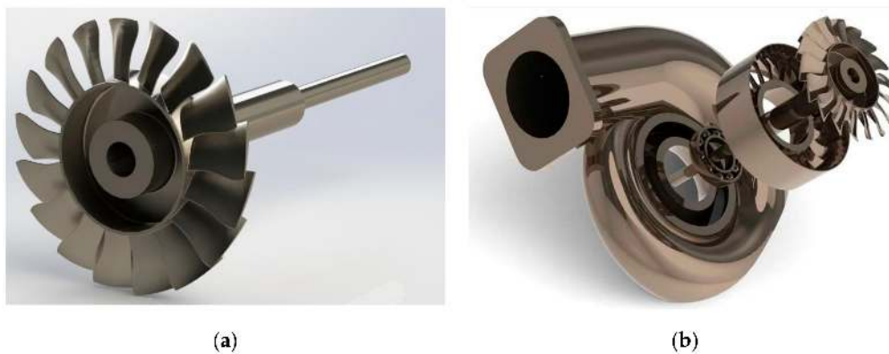
Figure 33. (a) Optimized blade design and (b) 3D model of the axial turbine.
