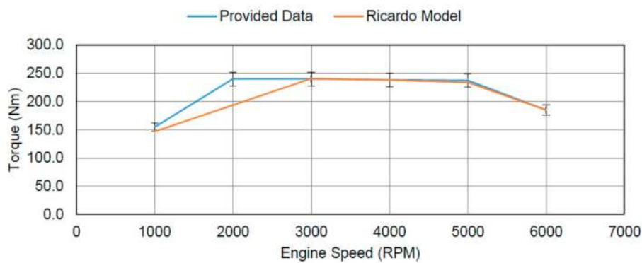
Figure 13. Comparison between provided engine torque and Ricardo WAVE model.
