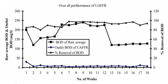
Figure 3 | Performance of UAFBR operation in BOD removal. (UAFFR in figure denotes UAFBR).
