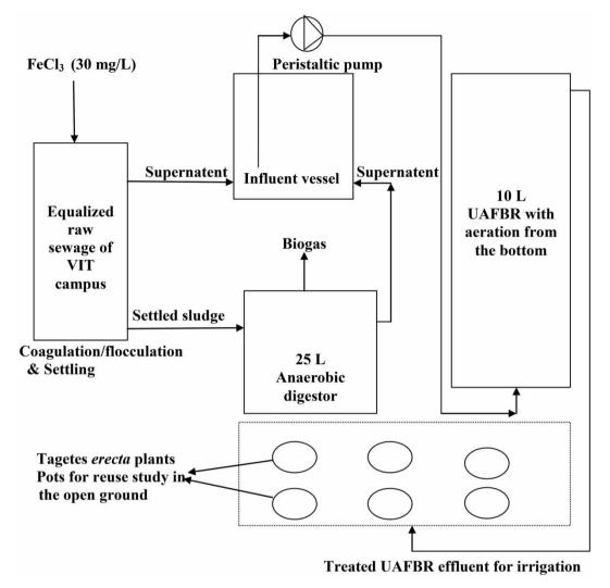
Figure 1 | The schematic of the lab-scale decentralized wastewater treatment system.
