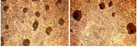
Sample 3(100X) processed at 350°C, 1hr Sample 4(100X) processed at 350°C, 2hr
