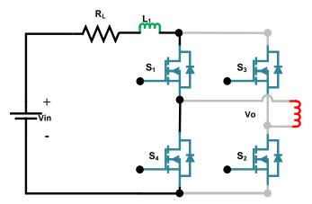
Figure 3. Current flow when  $S_1$ ,  $S_2$ ,  $S_3$ ,  $S_4$  are ON
