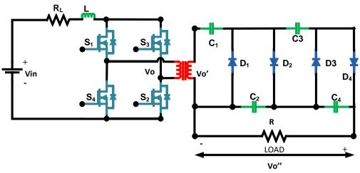
Figure 1. Isolated current fed boost converter topology
