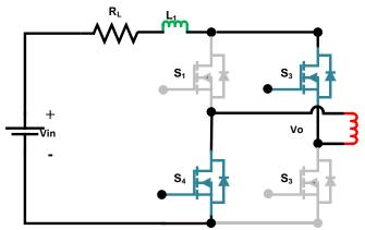
Figure 4. Current flow when S<sub>2</sub>, S<sub>4</sub> are ON
