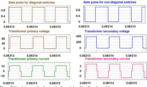
Figure 7. Simulation results of gate pulse for switches, V<sub>pril</sub>, V<sub>sec1</sub>, I<sub>pril</sub> and I<sub>sec2</sub>.
