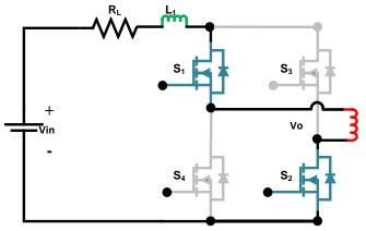
Figure 2. Current flow when  $S_1$ ,  $S_2$  are ON
