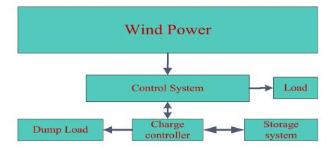
battery backup system. When the hybrid system generated power is in surplus, this power is used for loading the batteries for backup security and this charge battery power is used when the load requirement is not supplied by design hybrid system (Elhadidy & Shaahid, 2000). Figure 3 shows the architecture of wind hybrid energy system and Table 2 shows the summary of studies based on wind hybrid system.
