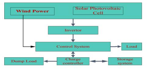
Figure 4. Architecture of PVwind hybrid system.
