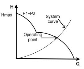
(d) Resultant performance curve with system curve (Dissimilar pumps)
