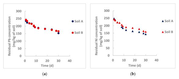
**Figure 5.** Remediation of nZVI particles synthesized using neem leaves (dosage: 0.2 g/kg of soil): (a) lead removal; (b) nickel removal.
