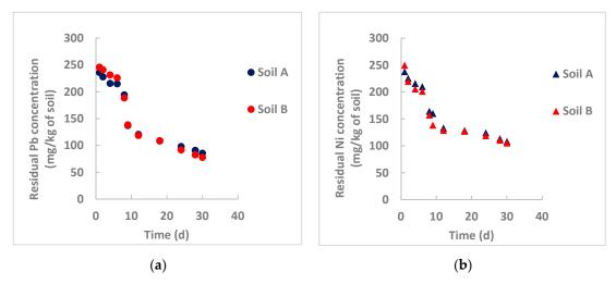
**Figure 7.** Remediation of nZVI particles synthesized using mint leaves (dosage: 0.2 g/kg of soil): (a) lead removal; (b) nickel removal.
