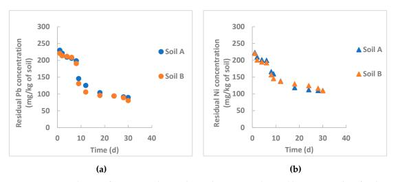
**Figure 6.** Remediation of nZVI particles synthesized using mint leaves (dosage: 0.1 g/kg of soil): (a) lead removal; (b) nickel removal.
