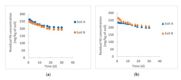
**Figure 3.** Remediation of contaminated soil using chemically synthesized nZVI particles (dosage: 0.1 g/kg of soil): (a) lead removal; (b) nickel removal.
