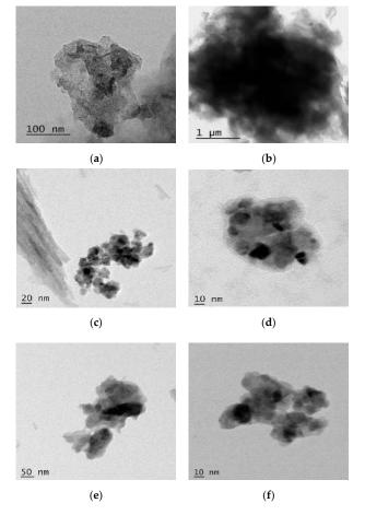
Figure 2. TEM image of nZVI particles: (a,b) chemically synthesized; (c,d) using neem leaves; (e,f) using mint leaves.
