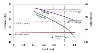
Fig. 5. Variation of voltage and frequency at different Loads.
