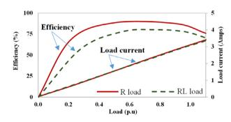
Fig. 3. Efficiency and current profile of synchronous generator.
