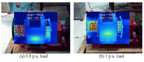
Fig. 6. Temperature variation under reduced dump load and full dump load in °F.
