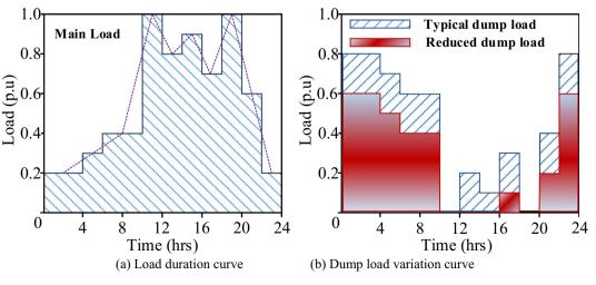
Fig. 9. Typical load curve of a micro hydropower plant.
