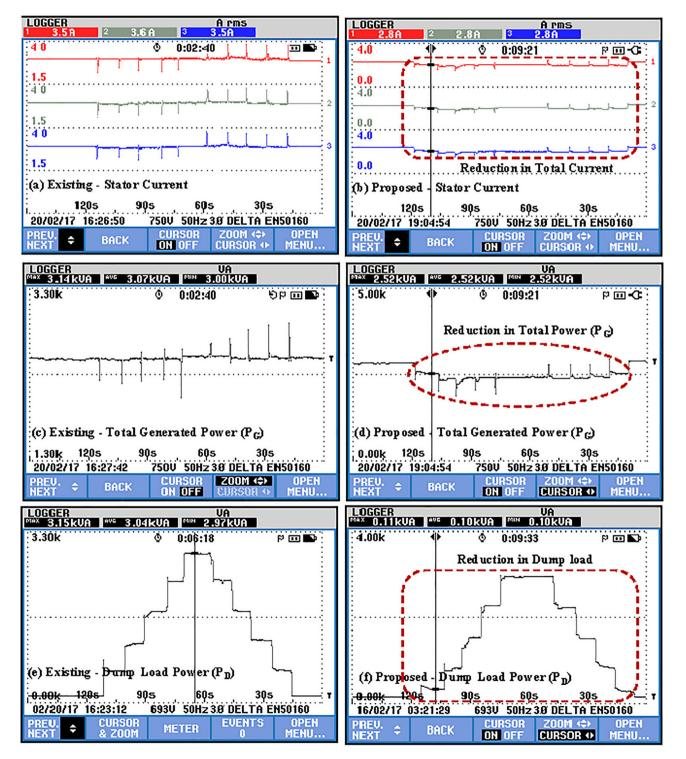
Fig. 12. Output electrical parameter of generator between existing and proposed strategy Existing - (a) Current; (b) Main Load power; (c) Dump load power Proposed - (b) Current; (d) Main Load power; (f) Dump load power.
