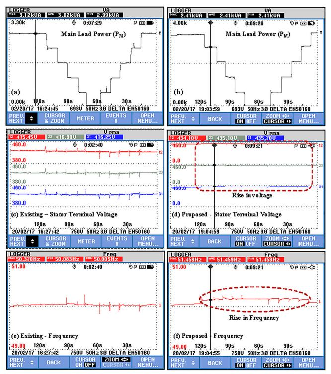
Fig. 11. Output electrical parameter of generator between existing and proposed strategy Existing - (a) Power; (c) Voltage; (e) Frequency Proposed - (b) Power; (d) Voltage; (f) Frequency.
