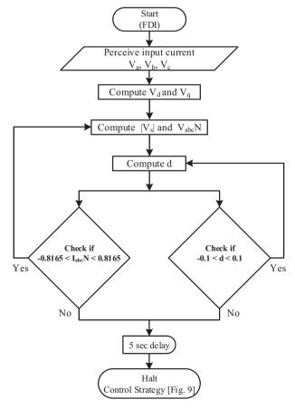
Fig. 7. Flow diagram for sensor fault detection and isolation.
