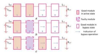
Fig. 14 Fault bypass operation and redundancy of MMC [100]
