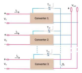
Fig. 18 Redundant leg implementation depends on simple redundant switch [40]
