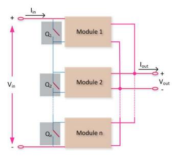
**Fig. 15** Fault-tolerant implementation in input series output parallel converter [102, 103] ( $Q_1$ ,  $Q_2$ ,  $Q_n$  denotes the bypass switches)
