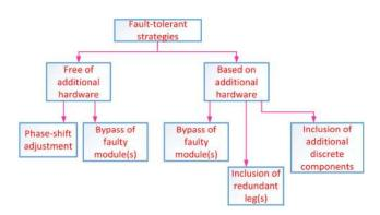
**Fig. 11** Categorisation of fault-tolerant strategies available in literature for DC–DC converters
