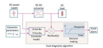
**Fig. 10** *Development of model-based fault diagnostic algorithm for DC–DC converters*
