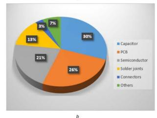
**Fig. 1** *Stress distributions and failure in power electronic systems* [6, 7] *(a)* Source of stress distribution, *(b)* Failure root cause distribution
