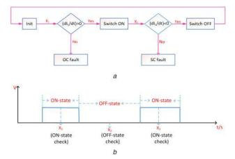
Fig. 5 Flowchart and gating signals [43](a) Flowchart accompanied by the state machine, (b) Gating signals v and instants
