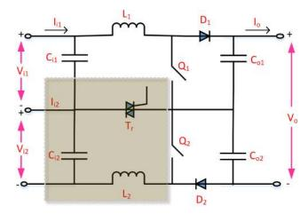
Fig. 17 Three-level boost converter fault-tolerant structure [44] (grey emphasise box includes new components establish in three-level boost converter)
