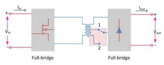
Fig. 16 FTO of full bridge DC–DC converter depends on auxiliary winding connected in secondary winding of transformer [39]
