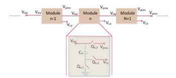
Fig. 13 Bidirectional MMC Fault-tolerant structure [99]
