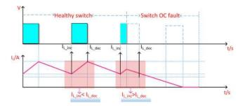
Fig. 6 Inductor current evolution in non-isolated unidirectional buck converter, under healthy and faulty conditions
