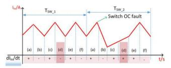
Fig. 8 Development of input current in time for 3-phase interleaved boost converter in two switching intervals. Highlighted the OC fault by shadowed portions during the  $T_{SW_2}$  period [51]
