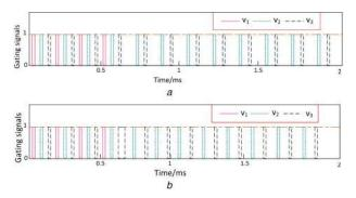
**Fig. 12** Interleaved switching pattern after OCF at t = 0.55 ms (a) Without reconfiguration, (b) With phase shift reconfiguration
