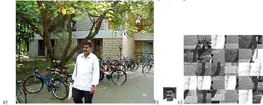
Fig.2. Target learning in initial frame a) Input 240x320; b) One Positive Sample 32x32: Class 1; c) Thirty Negative Samples 32x32x30: Class 0
