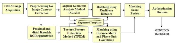
Figure 1 Block diagram of proposed personal authentication system.
