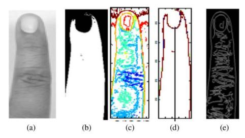
Figure 4 (a) Acquired FBKS image (b) binarized image of FBKS (c), (d) representation of contour extracted from binarized FBKS image. (e) Contour image of FBKS.
