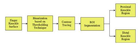
Figure 3 Block diagram illustrating ROI segmentation steps in personal authentication system.
