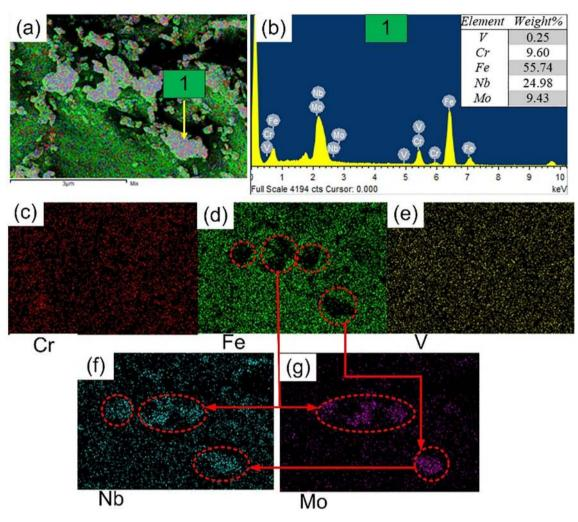
Fig. 9. For PWNT 2: (a) SE micrograph of WFZ with elemental mapping, (b) EDS spectra of precipitates, elemental mapping showing distribution of the: (c) Cr, (d)Fe, (e)V, (f) Nb, (g) Mo [34].
