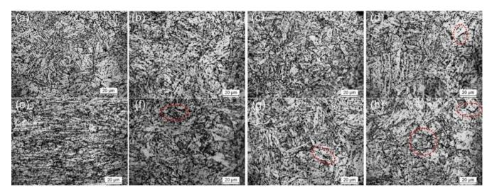
Fig. 2. Micrographs at different locations, as shown in Fig. 3(b); for PWNT 1 (a) at crack tip, (b) away from crack tip, (c) fine-grained HAZ, (d) WFZ; for PWNT 2 (e) at crack tip, (f) away from crack tip, (g) FGHAZ, (h) WFZ.
