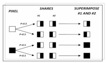
Fig. 1. Coding of Basic visual cryptography
