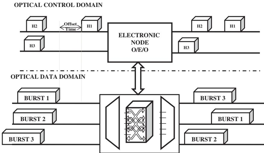
Figure 1: Core router architecture.
