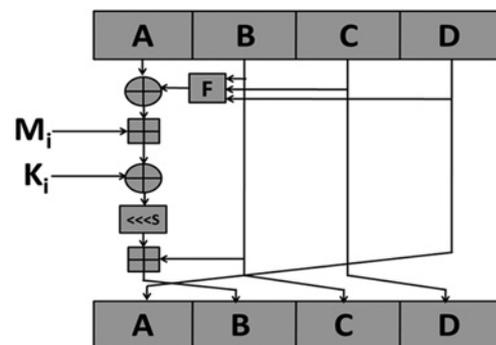
Figure 3: Modified MD5 algorithm.
