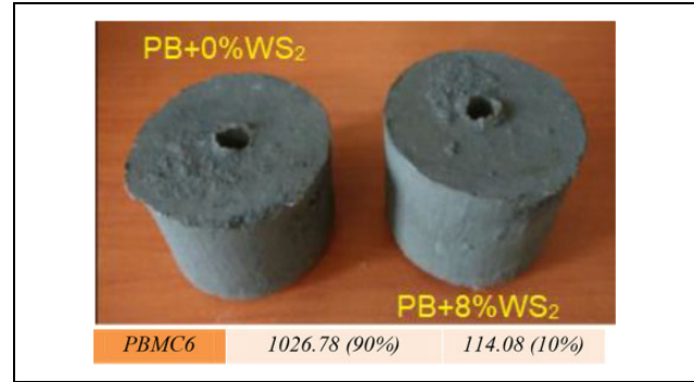
Figure 2. Composite samples fabricated for boring operation.
