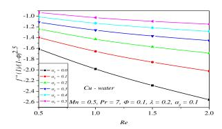
Fig. 13: Skin friction coefficient  $\frac{1}{(1-\Phi)^{2.5}}f''(1)$  under various values of Re &  $\alpha_1$ .
