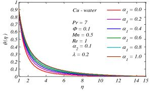
**Fig. 10:** Temperature profiles  $\theta(\eta)$  under various values of momentum slip parameter  $\alpha_1$
