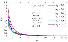
**Fig. 11:** Temperature profiles  $\, heta(\eta)$  under various values of thermal slip parameter  $lpha_2$
