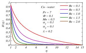
**Fig. 8:** Temperature profiles  $\theta(\eta)$  under various values of Reynolds number  $\operatorname{Re}$
