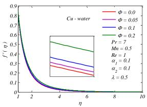
Fig. 5: Velocity profiles  $f'(\eta)$  under various values of nanoparticle volume fraction  $\Phi$  .
