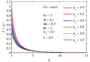
Fig. 9: Velocity profiles  $f'(\eta)$  under various values of momentum slip parameter  $\alpha$ .
