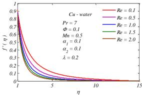
Fig. 7: Velocity profiles  $f'(\eta)$  under various values of Reynolds number  $\operatorname{Re}$ .
