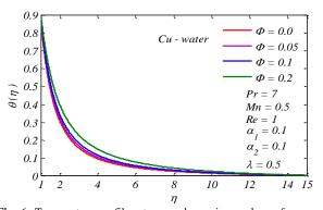
Fig. 6: Temperature profiles  $\theta(\eta)$  under various values of nanoparticle volume fraction  $\Phi$ .
