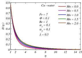
**Fig. 4:** Temperature profiles  $\theta(\eta)$  under various values of magnetic field parameter Mn.
