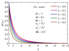
**Fig. 12:** Temperature profiles  $\theta(\eta)$  under various values of thermal relaxation parameter  $\lambda$
