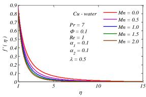
Fig. 3: Velocity profiles  $f'(\eta)$  under various values of magnetic field parameter Mn.
