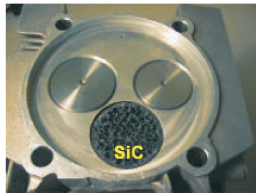
Figure 13. View of engine head with SiC ceramic material mounted in space between valves
