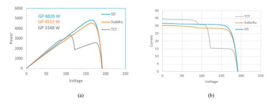
Fig. 4. (a) Case 1: PV Characteristics for TCT, SuDuKo and SDGA arrangements; (b) Case 1: IV Characteristics for TCT, SuDuKo and SDGA arrangements.
