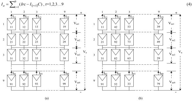
Fig. 2. Reconfiguration of PV array (a) TCT configuration scheme; (b) SuDuKo Configured PV Array.
