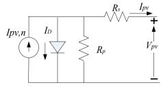
Fig.1. Schematic of One diode model.
