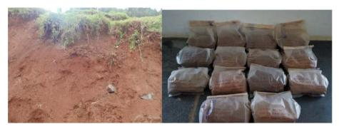
Fig. 1. a) Slope failed area from where soil is collected b) Soil samples.
