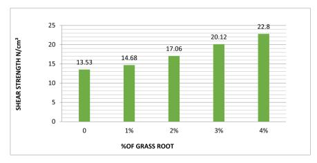
Fig. 7. The effect of Shear strength with the addition of various percentage of fibers.
