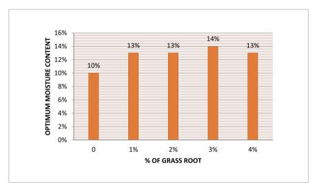
Fig. 6. The effect of OMC with the addition of various percentage of fibers.
