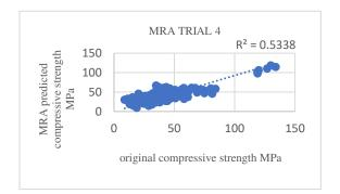
**Figure 7**. Original vs MRA predicted compressive strength (TRIAL 4).
