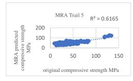
Figure 9. Original vs MRA predicted compressive strength (TRIAL 5).
