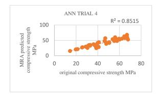
**Figure 8**. Original vs ANN predicted compressive strength (TRIAL 4).
