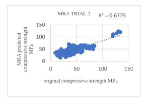
**Figure 3**. Original VS MRA predicted compressive strength (TRIAL 2).
