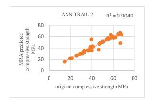
**Figure 4**. Original vs ANN predicted compressive strength (TRIAL 2).
