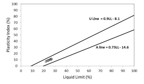
Figure 6. Plasticity chart for soil samples
