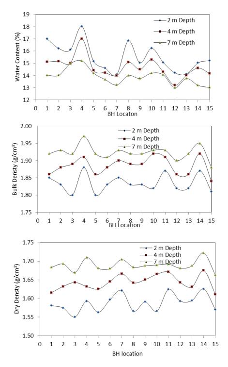
**Figure 3.** Variation of water content, in-situ bulk density and dry density with respect to depth of soil in different location of bore well (BH).
