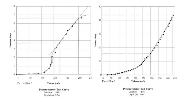
Figure 2. Pressuremeter test curves for BH1 at 7.5m & 11m depth
