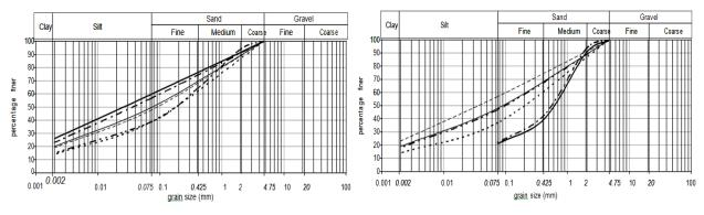
Figure 4. Grain size distribution curves for soil sample
