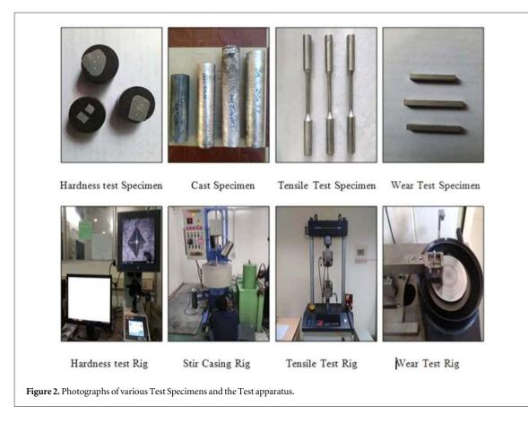
employed to test the tensile specimens. The failure analysis of fractured specimens was analyzed with the help of SEM images. Finally, the processed composites were tested for wear property with the help of Pin-on-Disc wear and friction testing Ducom equipment -TR 201 LE.
