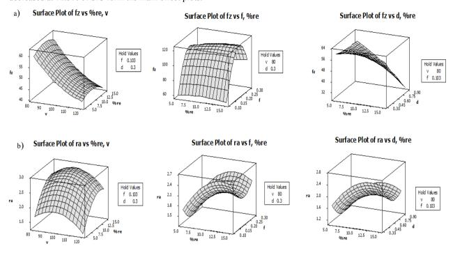
Fig. 4. Surface Plot of a) Cutting Force (Fz) and b) Surface Roughness (Ra)
