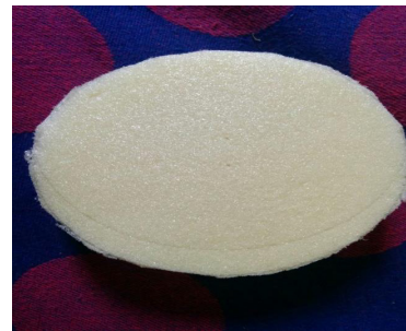
Figure 4. Rigid polyurethane foam in desire shape for impedance test.
