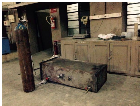
Figure 2. Carbonation chamber with CO 2 cylinder, CO 2 regulator and air heater
