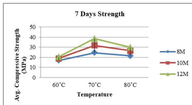
**Figure 2.** Compressive Strength at the age of 7 days curing
