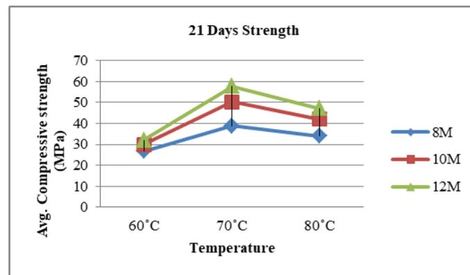
**Figure 3.** Compressive Strength at the age of 21 days curing
