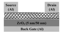
Figure 1: Cross-sectional view of SB CNTFET
