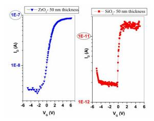
**Figure 7:** Comparison graph with different dielectrics. The plot in blue shows the characteristics for device with ZrO<sub>2</sub> (50 nm thickness) and plot in red shows the characteristics for device with SiO<sub>2</sub> (50 nm thickness)
