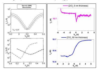
**Figure 6:** Comparison with the numerical simulation in Guo et al. [Guo, Datta and Lundstrom (2004)]. Left plot shows the IV characteristics of the numerical simulation in Guo et al. [Guo, Datta and Lundstrom (2004)]. Right plot is the IV characteristics for different gate oxide thickness (5 nm and 50 nm) of our experimental work
