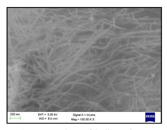
Figure 5: SEM image of the dispersed CNTs
