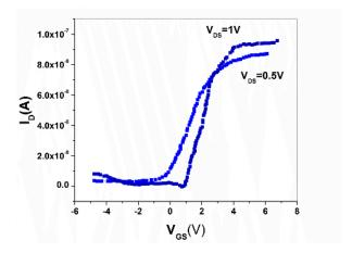
Figure 10: I<sub>D</sub>- V<sub>G</sub> characteristics of the device with thick gate oxide with suppressed ambipolar conduction
