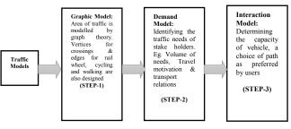
Figure 3. Architecture of traffic simulation model.
