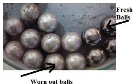
Fig. 1 Balls worn out after AA 2900 With SiC ball milled.
