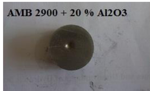
Fig. 5 Crack observed in Al 2 O 3 wt. 20%
