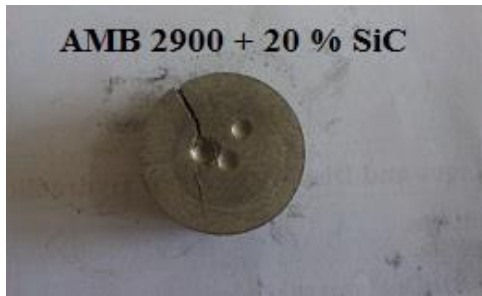
Fig. 4 Crack observed in SiC wt. 20%
