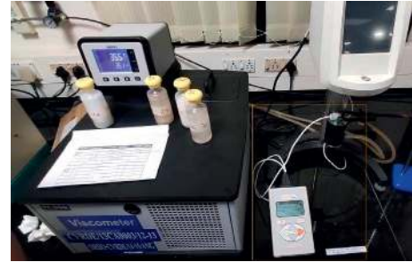
FIGURE 1: Experimental setup with viscometer and KD2 thermal property analyser.
