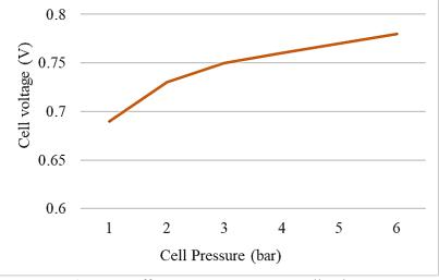
Figure. 5 Effect SOFC pressure on Cell voltage
