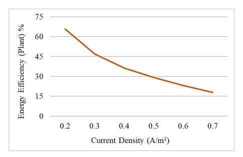
Figure. 2 Influence of current density on energy efficiency
