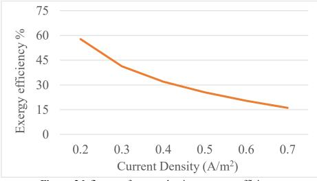
Figure. 3 Influence of current density on exergy efficiency
