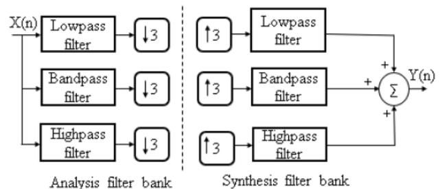
Fig. 2 Proposed three-tap biorthogonal wavelet filter bank
