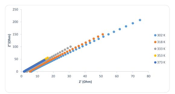
**Figure 3.4** Impedance diagram for PVdF-HFP(17.25)-PMMA(5.75)-LiClO<sub>4</sub>(8)-EC(69)-TiO<sub>2</sub>(10) at different temperatures
