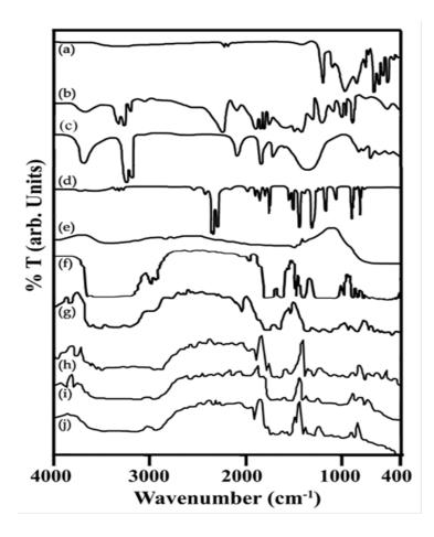
**Figure 3.2** FTIR Spectra of pristine material (a)PVdF- HFP(b)PMMA (c)  $LiClO_4$  (d) EC (e)  $TiO_2$  and (f-j) composite polymer electrolytes PVdF-HFP(17.25) PMMA(5.75)–LiClO<sub>4</sub>(8)- EC(69)-TiO<sub>2</sub>(X) [X=0 (f), 5 (g), 10 (h), 15 (i) and 20 (j)]
