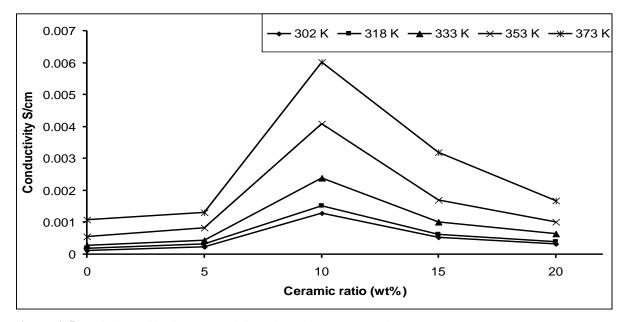
Figure 3.5 Variation of ionic conductivity with TiO<sub>2</sub> concentrations.
