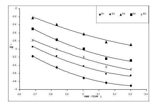
**Figure 3.3** Arrhenius plot of the conductivity for PVdF-HFP -PMMA -LiClO<sub>4</sub>- EC polymer complexes for TiO<sub>2</sub> (0,5,10,15,20 wt%) concentrations.
