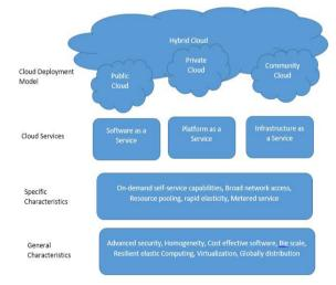
Fig. 1. The cloud computing model
