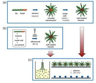
**Scheme 1.** The preparation of metal-salt-loaded micelles by conventional stirring (a) or by the new route based on ultrasonication in the presence of a co-solvent (b). After depositing micellar monolayers on top of appropriate substrates by dip-coating, ordered arrays of metal oxide or metal nanoparticles are obtained by applying oxygen/hydrogen plasmas (c).
