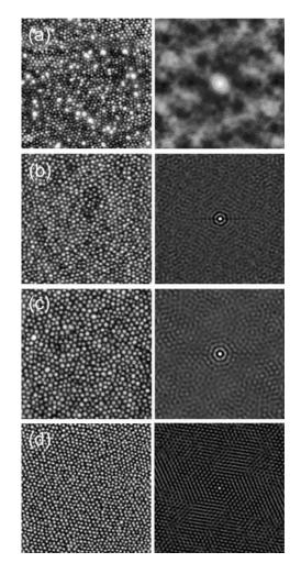
**Figure 1.** AFM results (left column) and related auto-covariance (right column) of iron-salt-loaded micellar monolayers derived from solutions prepared by a) conventional stirring for 1 week in the absence of any co-solvent; b) conventional stirring for 1 week in the presence of methanol; c) sonication for 60 s without additional co-solvent; and d) ultrasonication for 60 s in the presence of methanol (all images  $1 \times 1 \ \mu m^2$ ).
