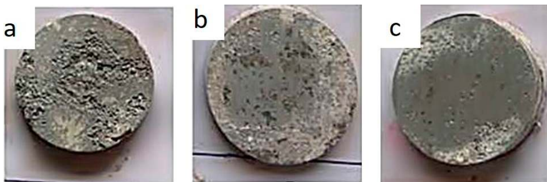
Figure 13. Surface macro-morphology images after salt spray test in 3.5% NaCl solution: (a) Acrylic paint ED coat; (b) 2-coat polyester without primer; (c) 3-coat polyester with epoxy primer.
