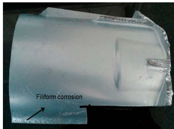
Figure 12. 3-coat polyester with epoxy primer.
